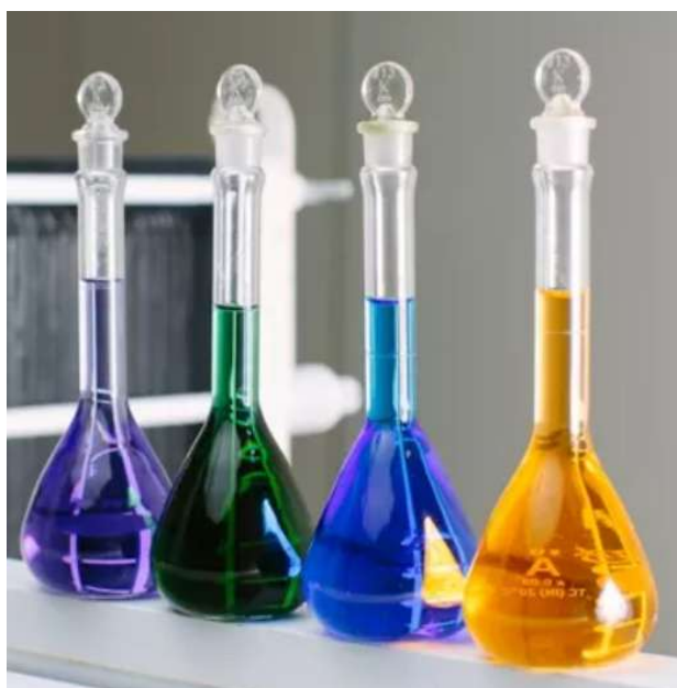
Figure 8.3 – Vanadium Electrolyte For Vanadium Redox Flow Battery VRFB 250 ( V^{3+} (green solution), V^{2+} (purple solution), VO^{2+} (blue solution), VO_2^+ (yellow solution))
