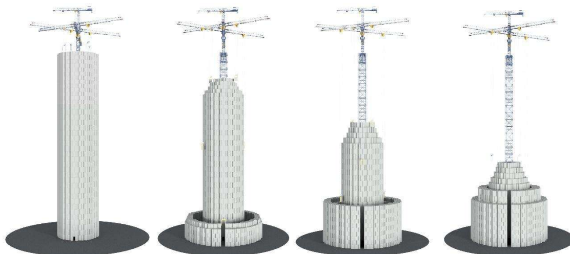
Figure 2.1 From left to right, Energy Vault's tower fully "charged," at partial levels of charge, and with its capacity fully expended. Source: Energy Vault 22
